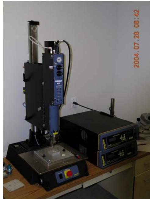
Figure 8 Ultrasonic Welder
