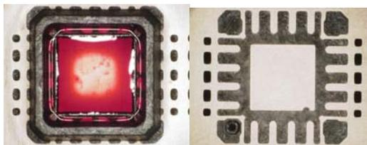
**Figure 3: Hermetic Plastic Package from QLP using Quantech™ (No leakage from Red Die)**
