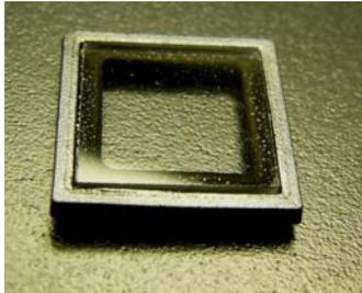
**Figure 6: Glass Lid embedded in Quantech™ ring**
