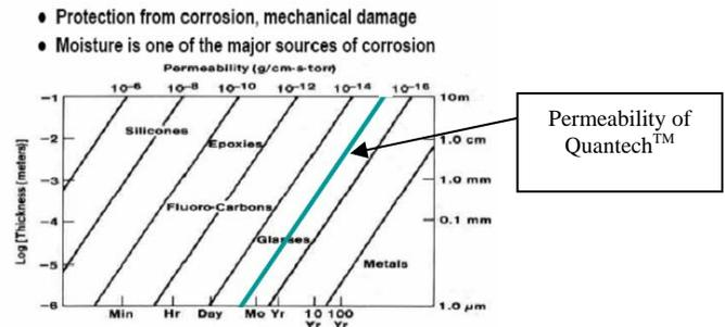
**Figure 2: Permeability of various materials with Quantech™**
