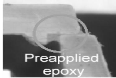
**Figure 4: Cross section of Lid attach using Epoxy**
