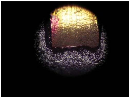
**Figure 1: Die Leaking Through Conventional LCP Package (Non Hermetic)**
