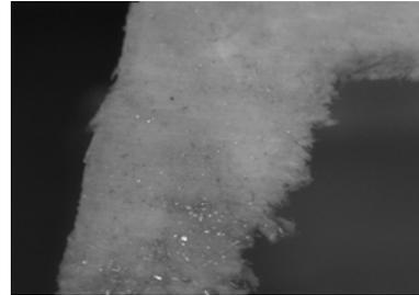
**Figure 5: Cross section of Lid Attach using UltraSeal™ Ultrasonic process**
