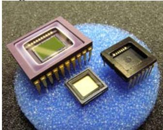
**Figure 7: Image sensor packages with glass lid and QLP Quantech™ Package**
