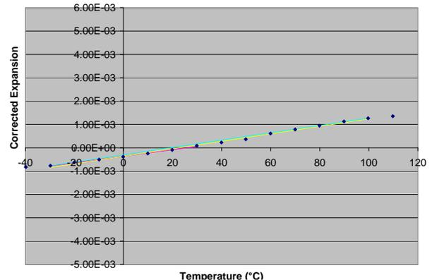
Figure 1: CTE of Novel Thermoplastic LCP in Flow Direction,  $17 \times 10^{-6}/^{\circ}\text{C}$
