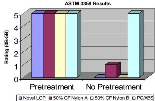
Figure 11: Paint Adhesion vs. Material
