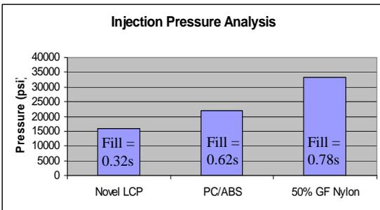
Figure 10: Injection Pressure vs. Material
