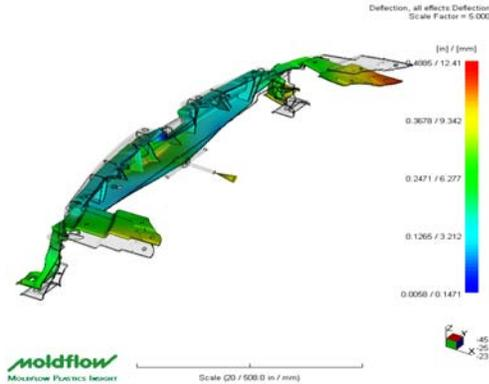
Figure 7: Mold Flow Analysis of the Novel Thermoplastic LCP
