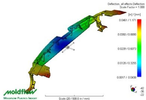
Figure 6: Mold flow Analysis of Glass Filled Nylon
