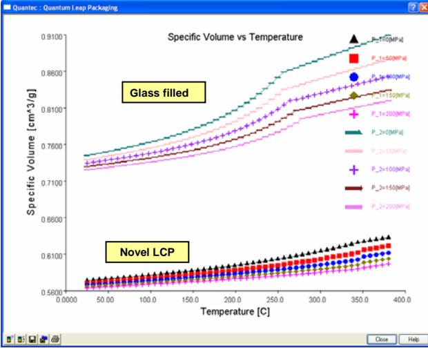
Figure 9: Specific Volume vs Temperature
