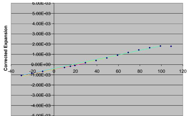
Figure 2: CTE of Novel Thermoplastic LCP in Cross Flow Directions,  $15 \times 10^{-6}/^{\circ}\text{C}$
